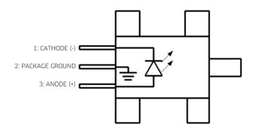
The anode and cathode of the laser will be in a floating configuration, i.e., the two pins will be isolated from the package ground with a resistance greater than 1  $M\Omega$ .
