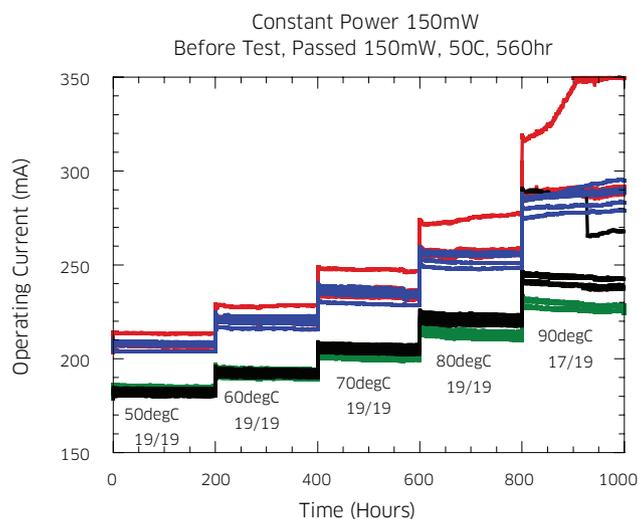
Fig. 1. Step stress test data on 810-850nm single-mode AlGaAs diode lasers (different colors represent different wafer material). Devices maintain 150mW operating power with no noticeable degradation to at least 70°C.
