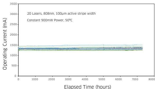
Fig. 2. Accelerated lifetest data for 100µm 808nm pump lasers showing negligible wear-out degradation and zero failures over 170,000 device hours. A conservative MTBF<sup>3</sup>175,000h is estimated for normal rated 1.2W, 25°C operation.
