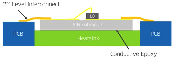
Figure 2: Bond wires are recommended for the interconnection between CoS and PCB
