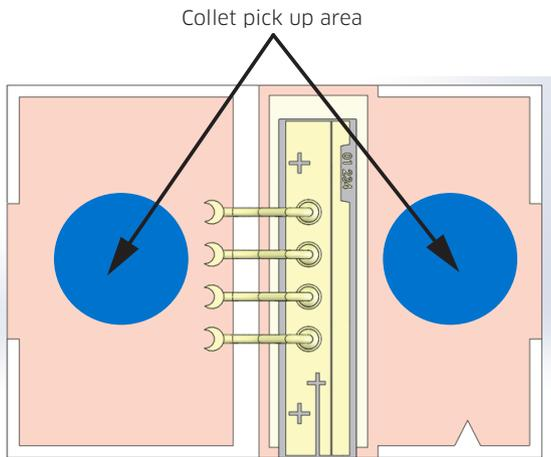
Figure 1: Each collet pick-up area highlighted in blue should have a maximum diameter of 0.25 mm
