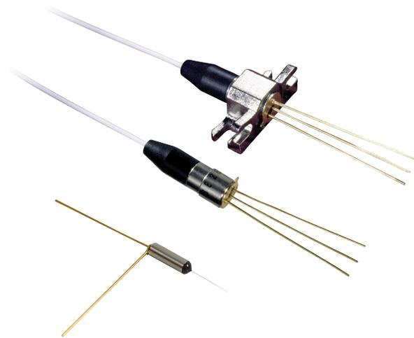
Lumentum EPM 6xx-Series PIN photodiodes are designed for optical network monitoring applications. The photodiode die is fabricated with a proprietary InGaAs process in our wafer fab and assembled into a hermetically-sealed package with antireflective-coated lens. A stainless steel bushing actively couples the fiber to the package.
