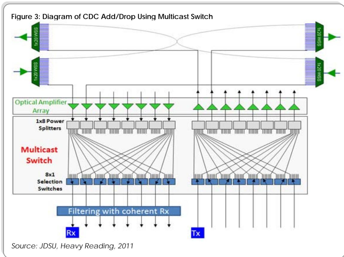
Initially, there was some interest in using larger-scale optical space switches (OXC) to deliver the add/drop flexibility required by CDC, but over the past year this interest has waned as these switches are relatively large and costly. Another gating factor for OXC has been the lack of support for flexible spectrum. Currently, the multicast switch architecture described above is preferred among equipment manufacturers.
