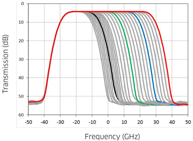
Programmable optical channel width supports 37.5 GHz, 50 GHz, 75 GHz, or any arbitrary channel width
