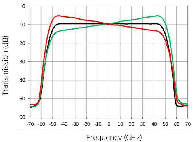
The TrueFlex WSS enables flexible intra-channel attenuation control for line power control and superchannel power balancing
